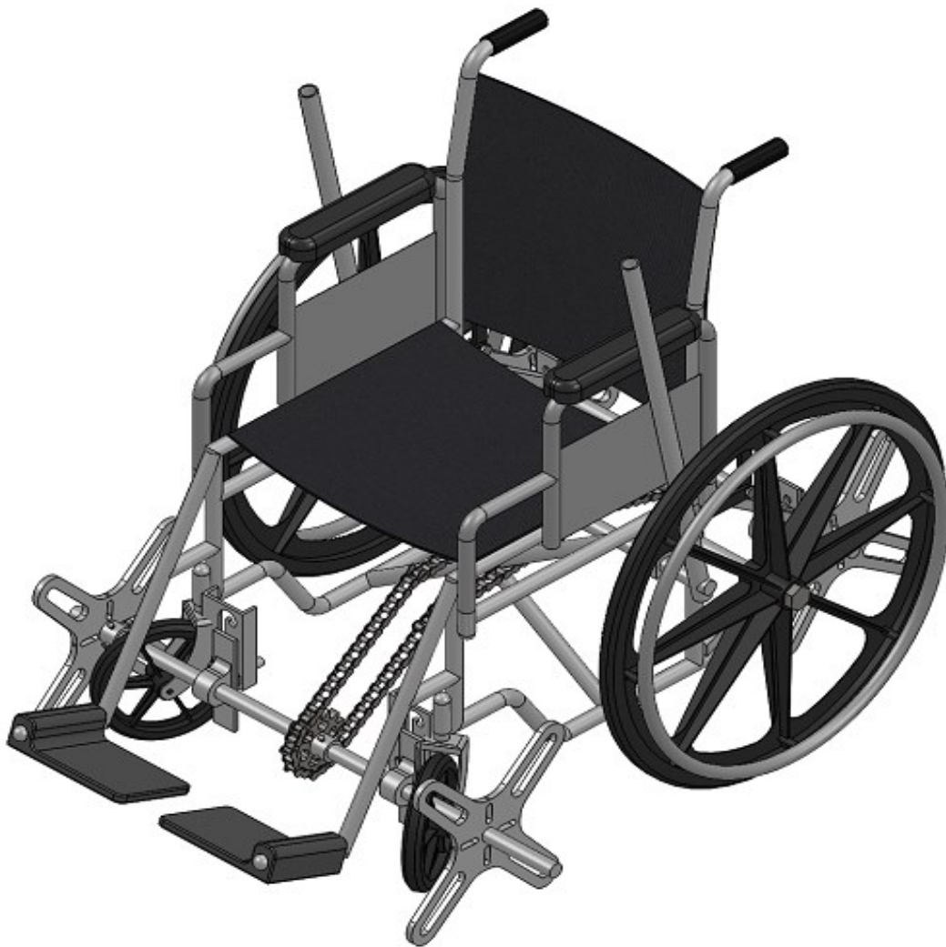
Figure: Stair Climbing Wheel Chair (Isometric View)
