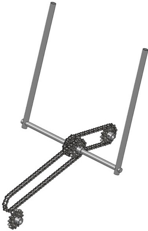
Figure: Middle Stair Climbing Assembly (Isometric View)
